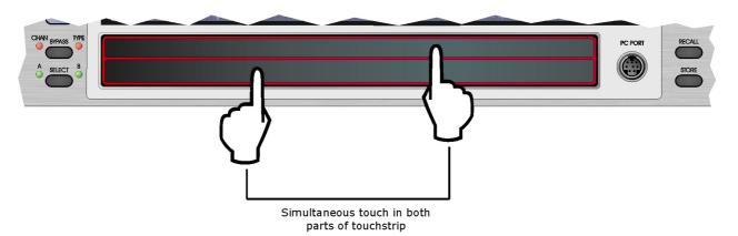
Groups of faders can be created and moved together. This is achieved by pressing below one fader on the upper strip, and below a different fader on the lower strip. A group will be created that includes all faders between those two selected ones. This can now be moved up and down using the encoder knob or by using the touchstrip in the area below the group. Pressing the touchstrip outside the range of the group or moving the "frequency" encoder knob will disband the group.
